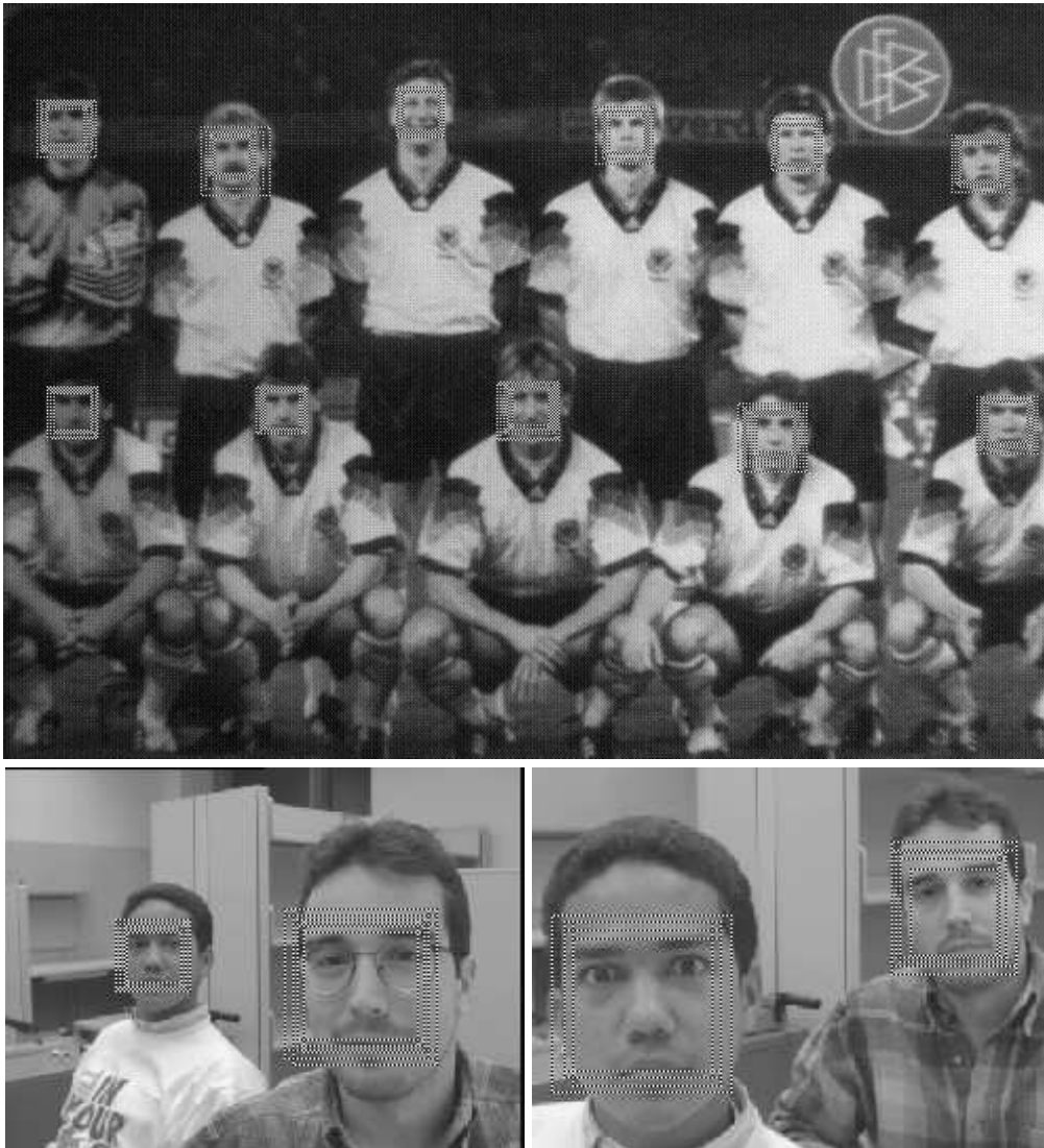
Figure 3.22: Face recognition example. Faces are extracted from an image of the German soccer team and two lab images. Copyright © 1997 [Osuna et al., 1997].
